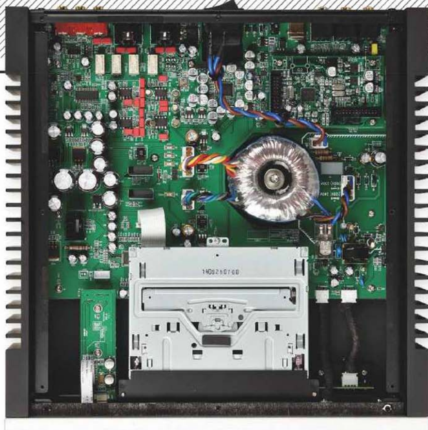
ABOVE: A slot-loading CD mech, plus S/PDIF and DSD-compatible USB ins, feed a balanced analogue stage based around the ESS Sabre ES9018 8-channel DAC, used here in dual-differential mode
