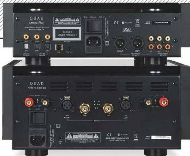
ABOVE: The Artera Play [top unit] has two optical and two S/PDIF coaxial plus USB digital ins, a pair of analogue ins plus single-ended RCA and balanced XLR outputs. The Stereo power amp [lower unit] has balanced and unbalanced inputs with single sets of 4mm speaker posts. Both units seen here with their detachable top plates
